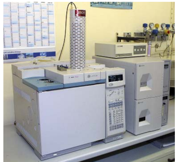
Fig. 1: Capillary gas chromatography coupled with a new ANTEK 7090N Nitrogen detector for analyses of NDMA
