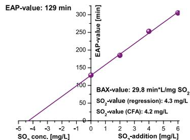
Fig. 6: BAX evaluation by linear fit of EAP values (BAX = slope).
