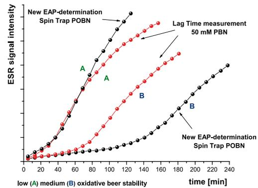
Fig. 2: New »EAP Determination« compared to conventional lag-time measurement.
