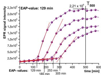
Fig. 5: ESR measurement of beer, EAP after SO<sub>2</sub>-addition 0,2,4,6 mg/L.
