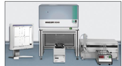
Electron spin resonance spectroscope
